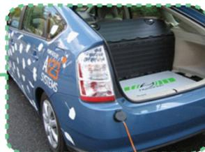
Reflecting the Prius' success, ubiquity and owner enthusiasm, a small after-market for converting the Prius to a plug-in develops; even dealerships offer to perform the conversion, which involves modifications to the software and installation of an outlet and larger battery.
